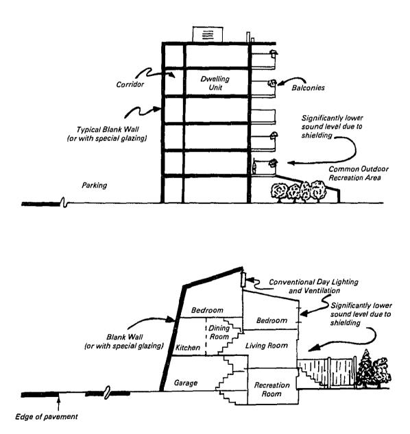
Figure 8, Designing Buildings to Attenuate Noise
